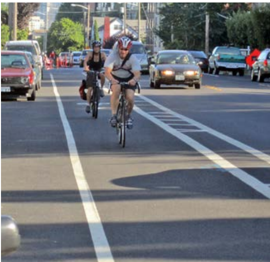
Figure 28 | Bike Lane — Buffered
