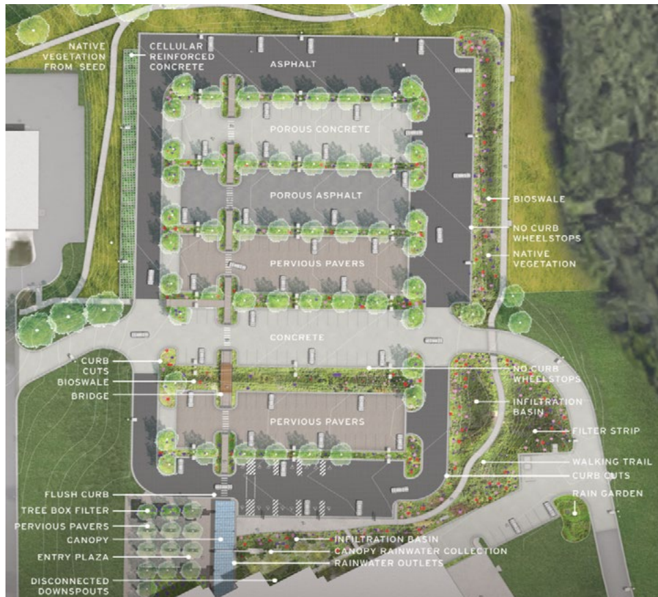
The Kansas City, Missouri Water Services Campus parking lot is a local precedent and resource for the installation, maintenance, and performance monitoring of multiple pervious pavement systems.
