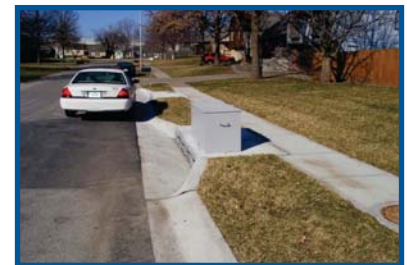
Temporary stormwater sampling box.
