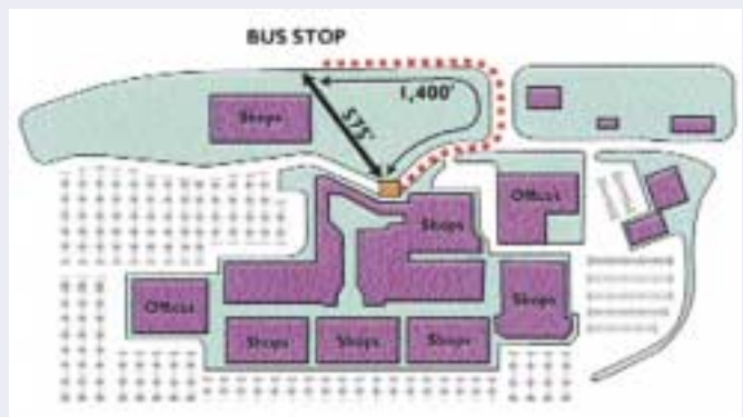
Walk time for a transit user is reduced with a direct connection to the bus stop
