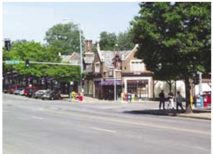
These valuable Kansas City area addresses are on streets designed with on-street parking, street trees and wide sidewalks, all of which buffer pedestrians from moving traffic.
