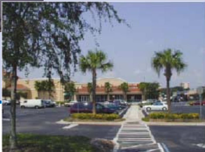
If large surface parking lots are necessary, walkways for through pedestrian traffic should be provided.
