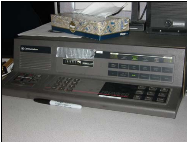
Factory Made RF Control Station (North KC PD’s KCMO EDACS unit)
