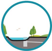
Temporarily store (**detain**) larger amounts of rainfall to reduce flooding and protect streams.
