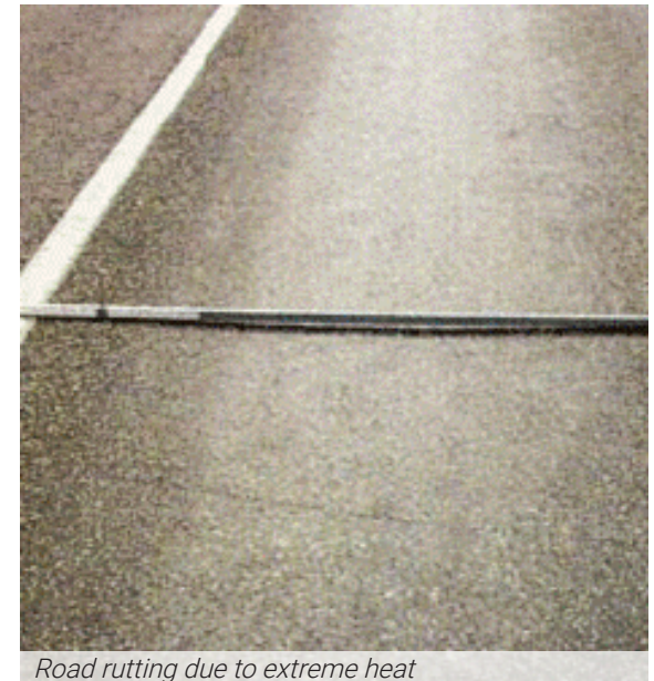
Road rutting due to extreme heat
