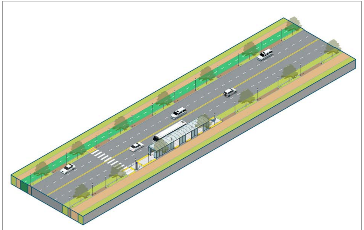
FIGURE 35: CROSS SECTION OF BRT-LITE AT STATION LOCATION
