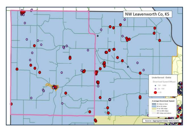
The ISPs in this area do not include any cable-to-the-home or fiber-to-the-home options. The fastest service (Mercury Broadband) has a fixed wireless option with a maximum advertised download speed of 100 Mbps and a maximum advertised upload speed of 20 Mbps. The remaining ISPs use fixed wireless, DSL, and satellite technologies and offer speeds less than 50 Mbps.
