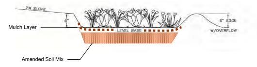
Typical Rain Garden Cross Section (Modified from Pennsyvania Stormwater BMP Manual, 2005)
