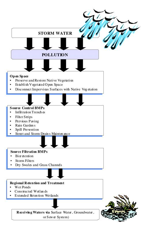
FIGURE 3.3 - Stages of a Treatment Train
