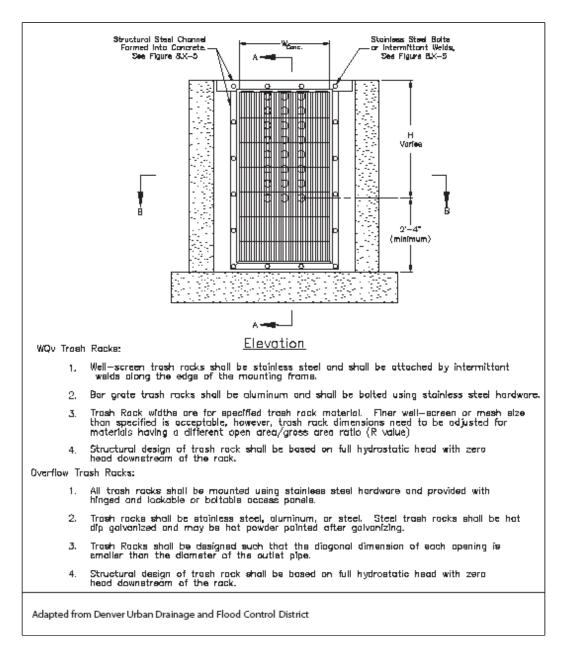
Figure 8.15 - WQv Outlet Trash Rack Design (2)
