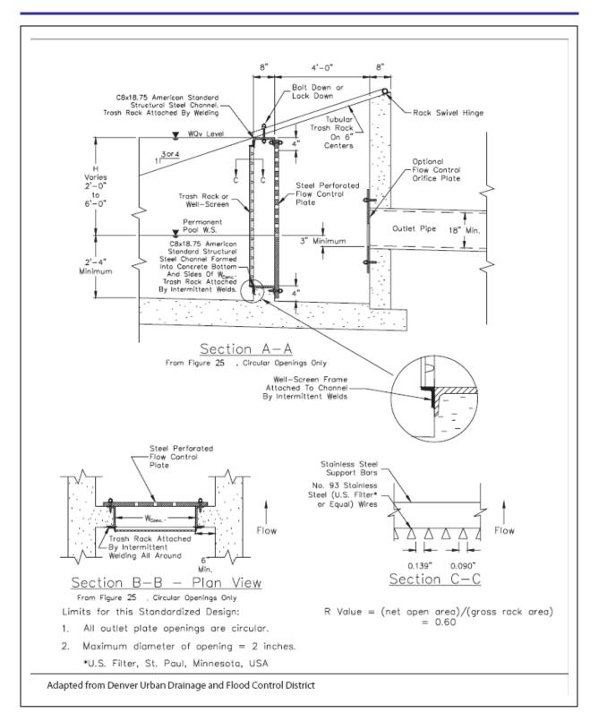
Figure 8.16 - WQv Outlet Trash Rack Design (2)
