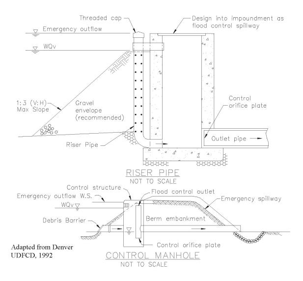
Figure 8.19 - Standpipe Outlet Structure
