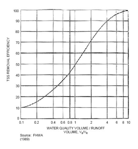
Figure 8.6 - TSS Removal Effciency of an EDW
