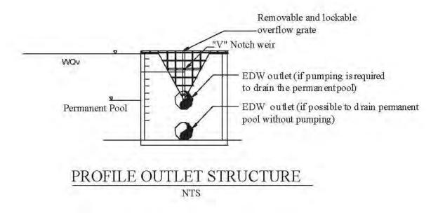
Figure 8.7 - "V" Notch Weir Outlet Structure
