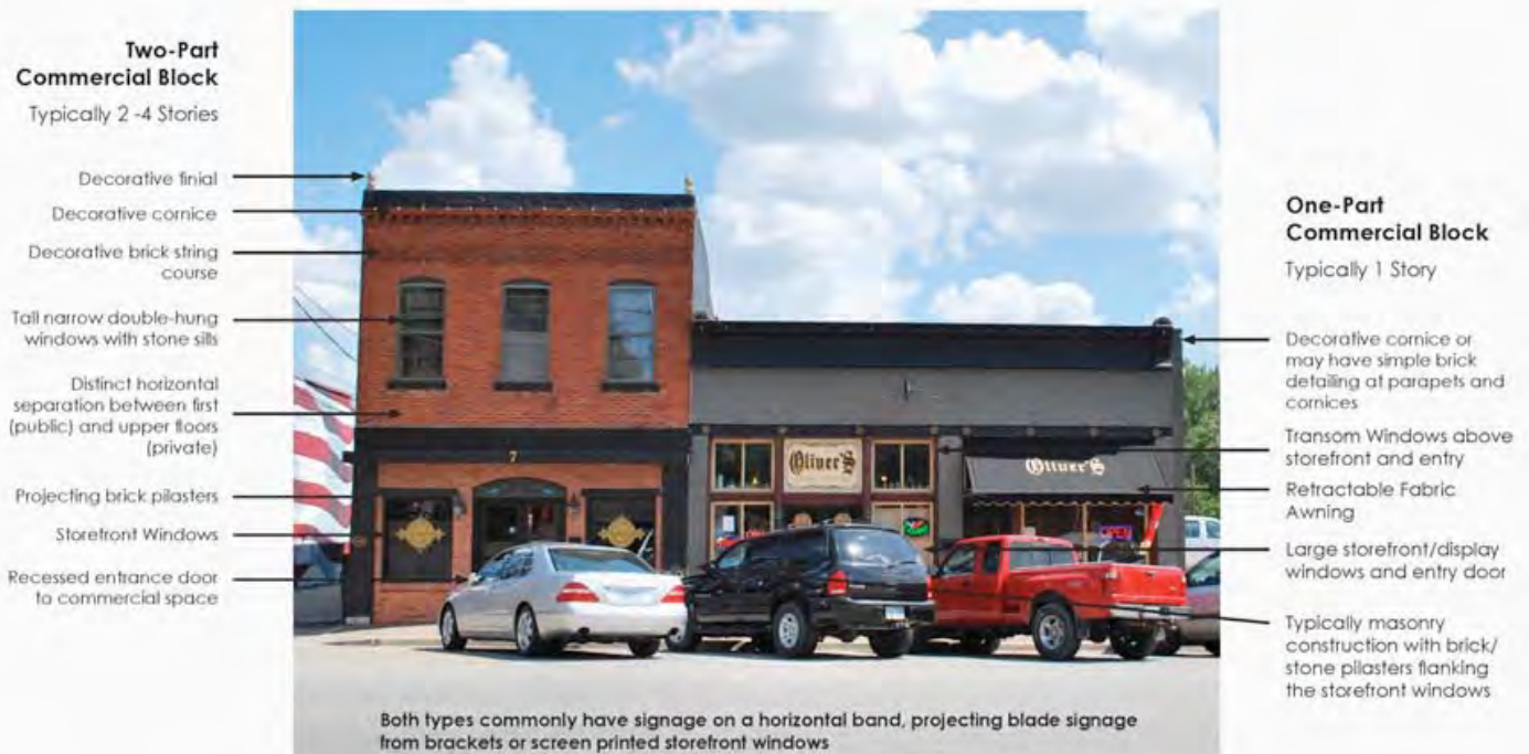
Fig. F.11 – Storefront terminology diagram. (SRJA, 2013).
