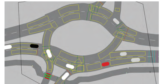
FIGURE 2.23 - SCREENSHOT OF CODING PROCESS THAT RESULTED IN FINAL VISSIM TRAFFIC MODELING CALCULATIONS
