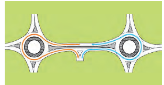
FIGURE 4.3 - ROUNDABOUT ACCESS MANAGEMENT (SOURCE: FHWA)
