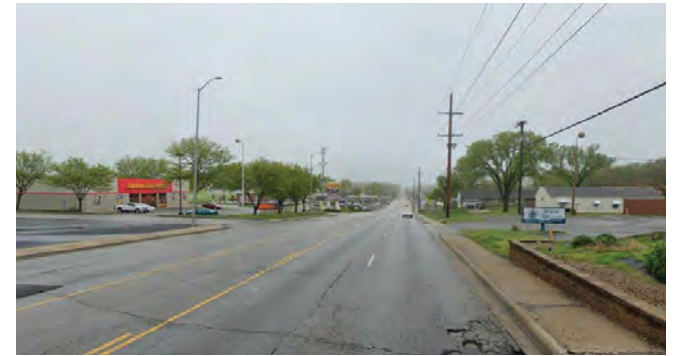
FIGURE 2.28 - SIDEWALKS CLOSE TO CURB AND LONG DISTANCES BETWEEN CROSSINGS RESULT IN LOW WALKING COMFORT
