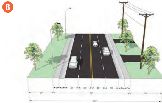
FIGURE 1.22 - EXISTING 4-LANE CONFIGURATION WITH INADEQUATE SIDEWALK CONDITIONS - 101' ROW
