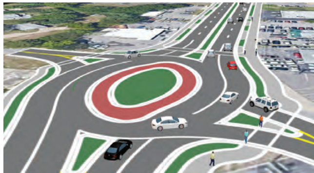
FIGURE 2.22 - A VISSIM MODEL WAS USED TO CALCULATE TRAVEL TIMES AFTER ROADWAY IMPROVEMENTS
