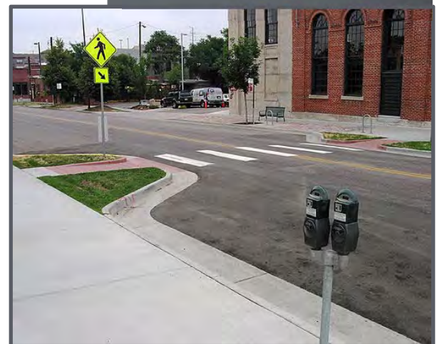
Figure 5.12: Mid-block crossing example with bulb-outs
