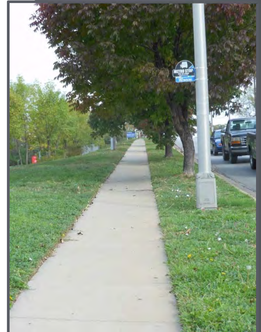
Figure 5.7: Vegetation strip with street trees separating pedestrians and traffic at North Oak, north of Vivion
