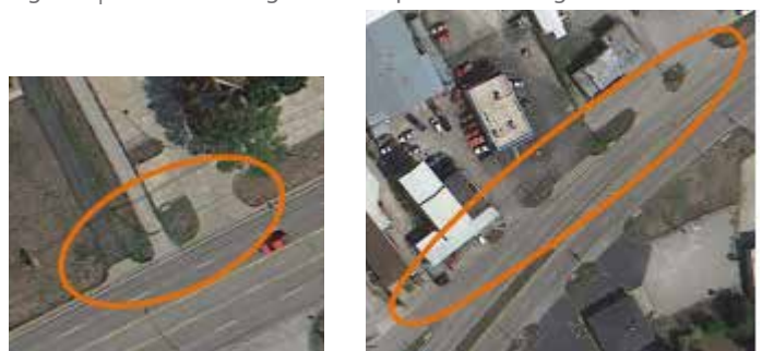
Figure 6 | These two images highlight areas with a high number of access points with very little separation. This is problematic throughout this segment of the corridor making traffic conflicts likely.
