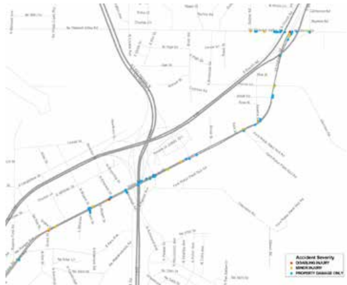
Figure 45 | Crash data by accident severity showing the locations where crashes were reported during a two year period between 2009 and 2011.
