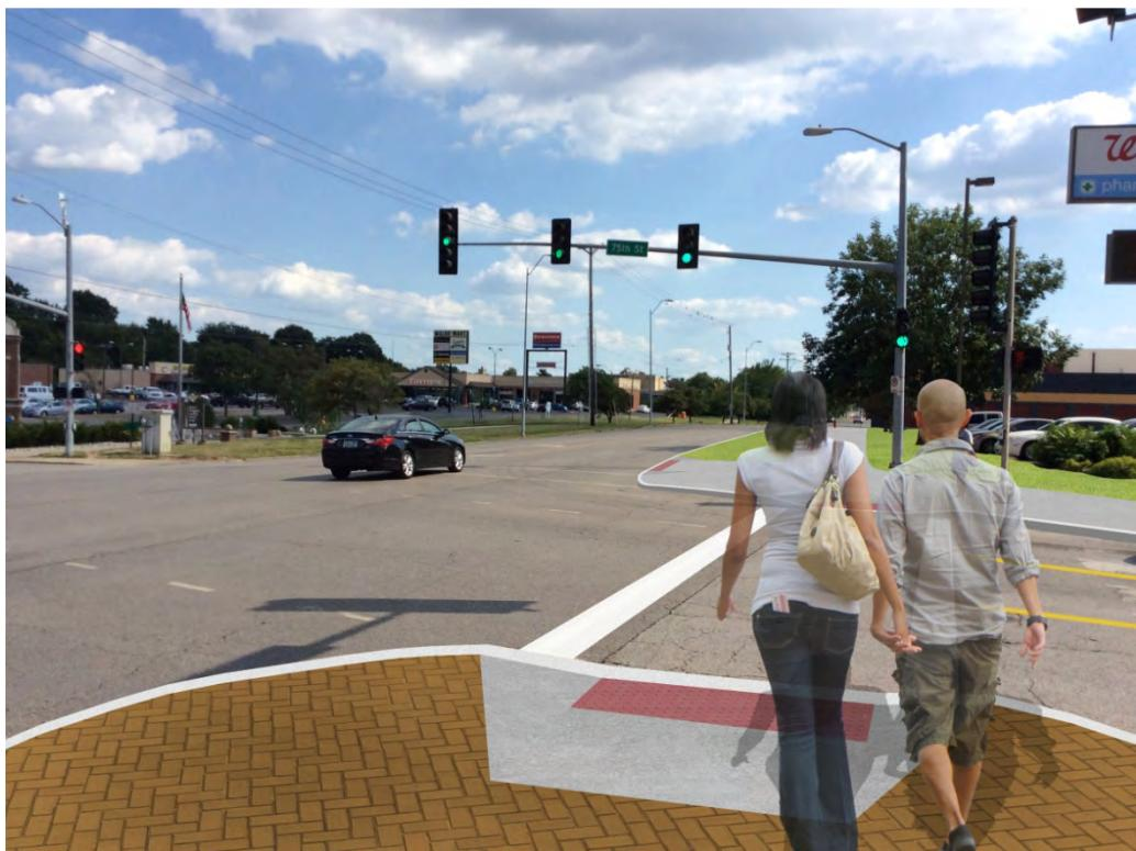
**Figure 10:** A proposed bump-out at 75th and Wornall, looking south, would reduce the roadway crossing distance for pedestrians and result in improved safety and aesthetics. Bulb-outs also calm traffic due to reduced lane widths.
