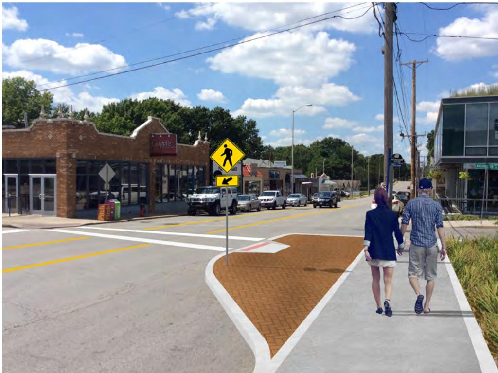
**Figure 9: A proposed bulb-out at 75th and Washington, looking west, would reduce the roadway crossing distance for pedestrians and result in improved safety and aesthetics. Bulb-outs also calm traffic due to reduced lane widths.**
