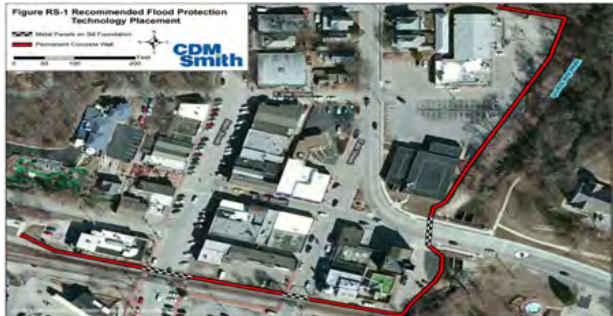
Figure RS-1 Recommended Flood Protection Technology Placement, as shown in the Flood Protection Study, December 2013
