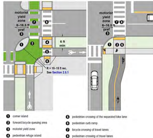
Figure 7-12: Protected Intersection Design for Separated Bike Lanes and Side Paths
